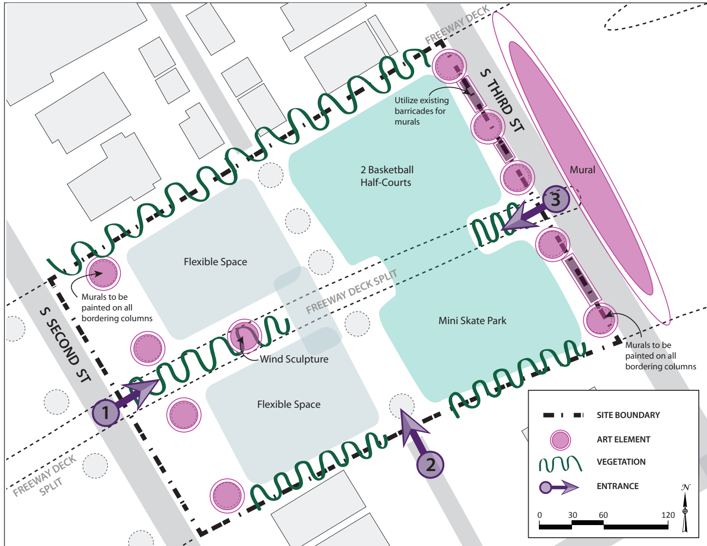
FIGURE 5.1 Conceptual design for the 2 nd & 3 rd Street/I-280 underpass
