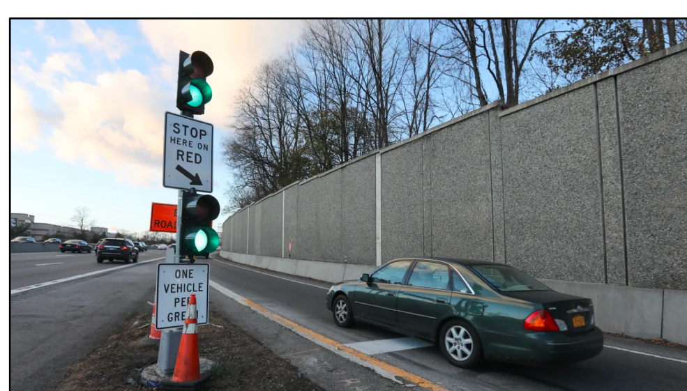
Figure 2: Example of Coordinated Ramp Metering system.
