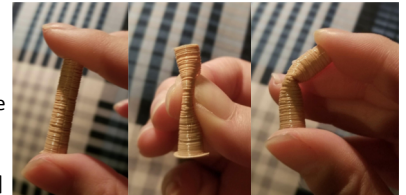
Figure 3 (Left). A prototype of the 3D printed PLA endoskeleton components were snapped together to form articulating joints capable of passive grasping [4]
