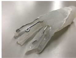
Figure 1 (Left). The Light Touch Hand prosthesis [2] facilitates passive grasping tasks, but has limited cosmesis. The Physolino Babyhand prosthesis [3] has a realistic appearance, but has no functional features
