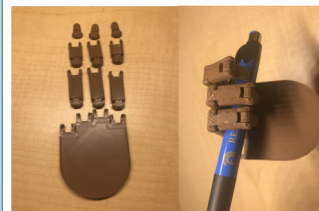
Figure 3 (Left). A prototype of the 3D printed PLA endoskeleton components were snapped together to form articulating joints capable of passive grasping [4]
