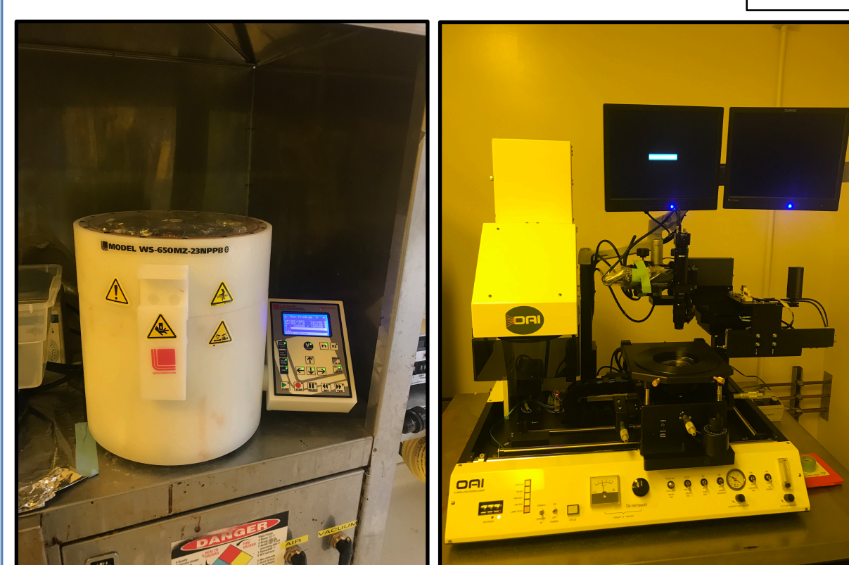
Figure 3. From Left to Right Spin coater and MEMS Mask Aligner/ UV Light Source. The spin coater covers the wafer with a negative photoresist layer, which is cured using a hot plate, and then placed in the aligner with the photomask on top. The photoresist is then exposed to UV light through the pattern on the mask. The resulting wafer with the negative photoresist design is then washed, leaving only the cured photoresist.
