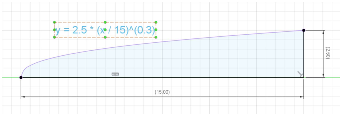
Figure 3.1 — Power series curve for nose cone design.
