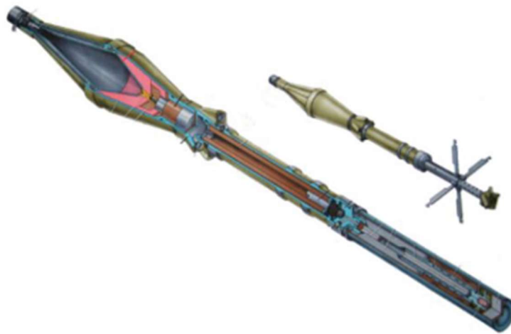
Figure 1.5 — PG-7 unguided rocket with stabilizer fins deployed [11].
