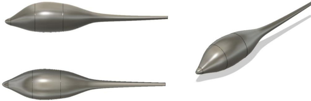
Figure 5.4: Front-view, top-view, side-view, and isometric view of the fuselage
