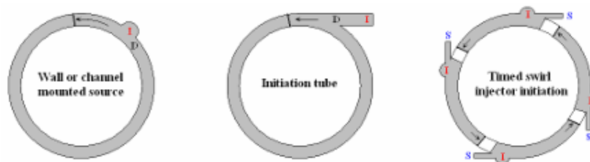
Figure 2.4 - Three different versions of RDRE detonation initiations. Diaphragm, initiation, and swirl are labeled D, I, and S respectively.
