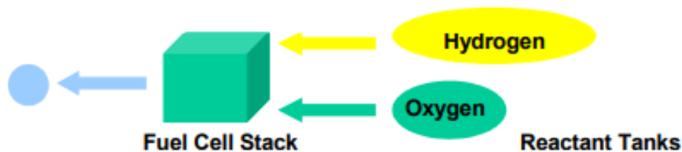
Figure 1.7 – PEM fuel cell diagram [14]
