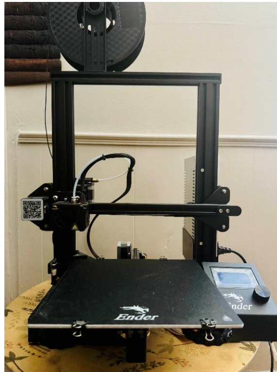
Figure 2.8 – Ender 3 3D printing setup.
