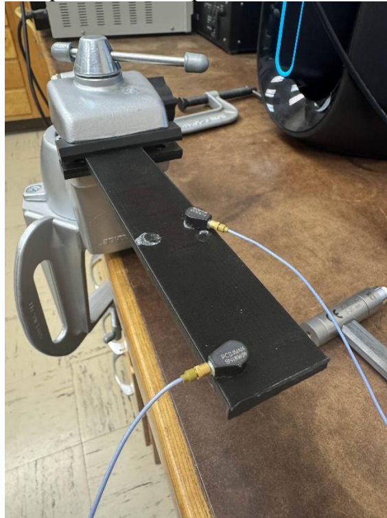
Figure 4.1 – Clamped 3D printed beam with accelerometers.
