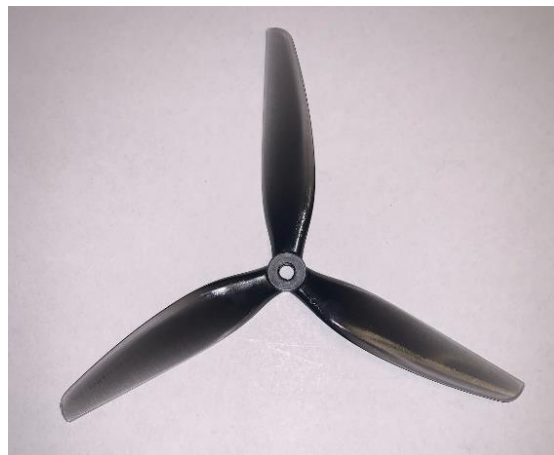
Figure 2.1. Chosen 7x4x3 inch Polycarbonate propeller.
