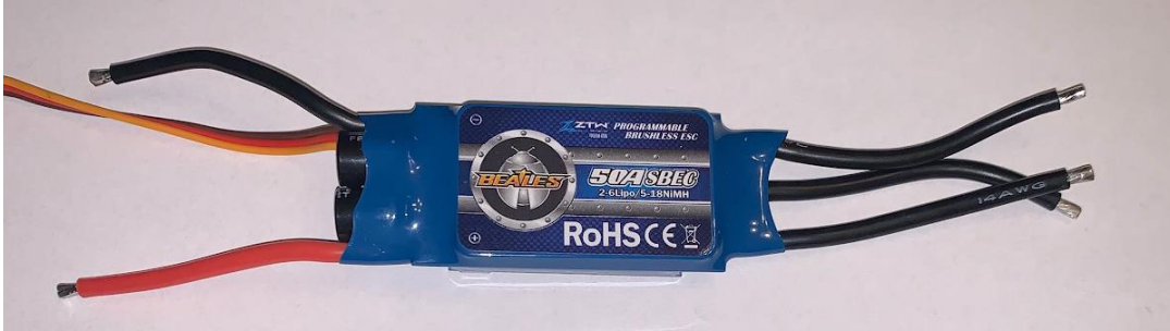
Figure 2.3. 60-Amp Brushless ESC chosen for the vehicle.
